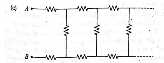
An infinite ladder network of resistances is connected across the points A and B, as shown in the above figure. Each of the resistance is  $1\Omega$ . Calculate the effective resistance between points A and B.
