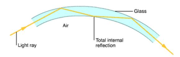
Optical Fiber are used to when high bandwidth, long distance, or immunity to interference is required. They have 3 components: Core made of glass; Cladding material surrounding the core; Outside coating
