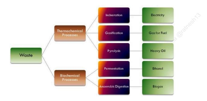
Pyrolysis is defined as a process of temperature decomposition of organic material in the absence of oxygen - syngas is produced
